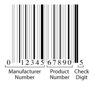
The 12-digit UPC barcode consists of three parts:
